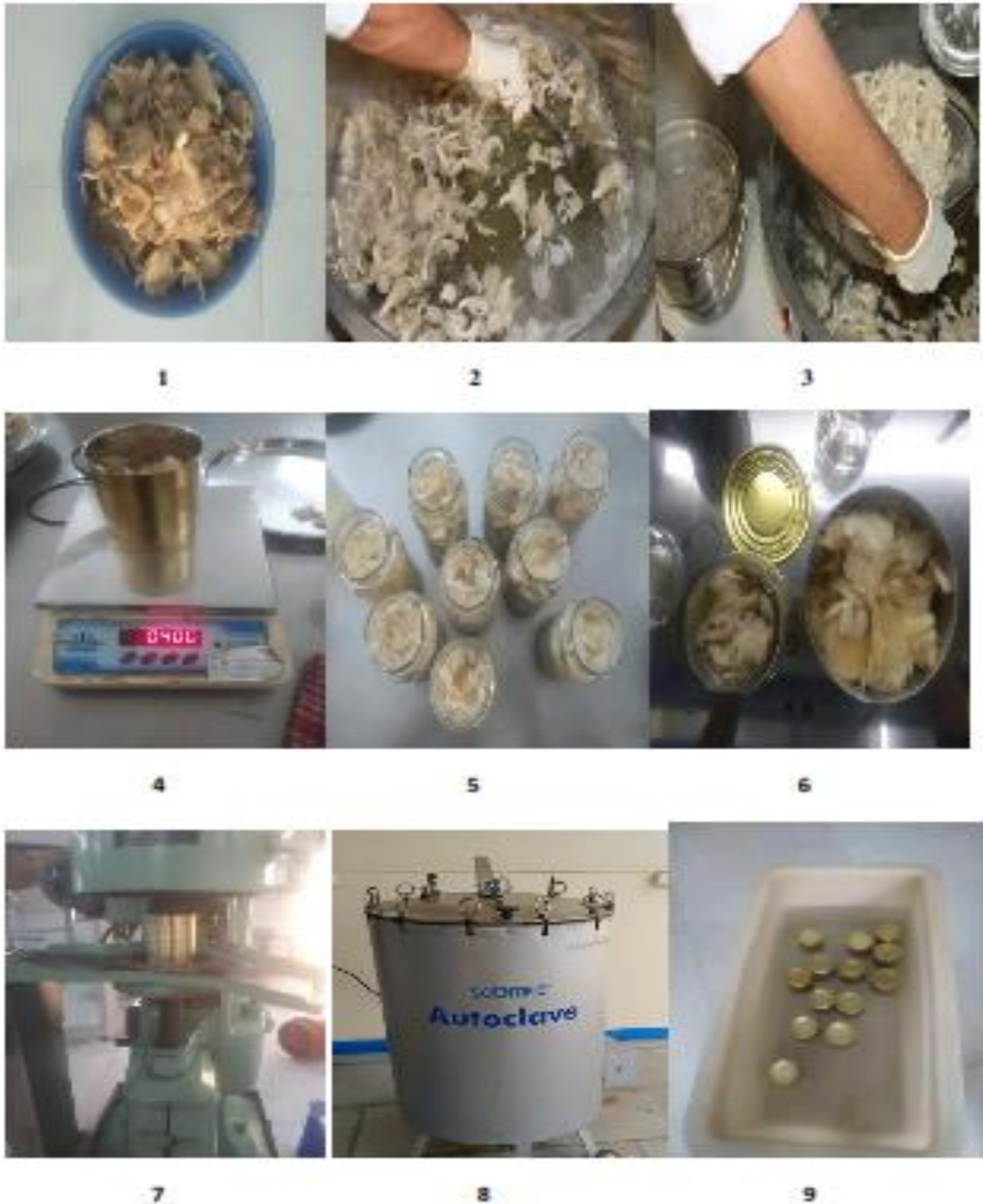
Figure 1: (1) Washed oyster mushroom, (2) Blanching (3) Water drain from blanched oyster mushroom (4) Weighing (5) Oyster mushroom bottles (6) filling in containers (7) Seaming (8) Retorting (9) Cooling.
